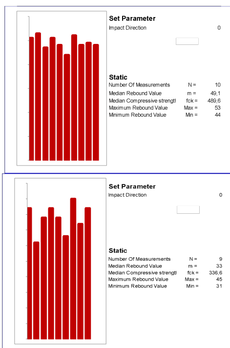
Figure 3. Sample of Hammer Test Results source: research data
