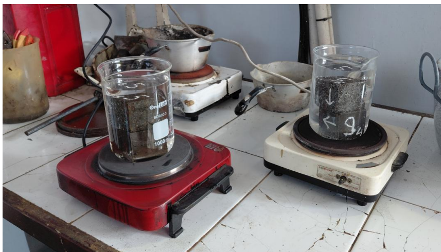
Figure 5. Boiling Process for Absorption Test Specimens
