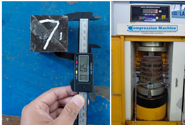
Figure 7. Measurement Process (Left) and Compressive Strength Testing (Right)
