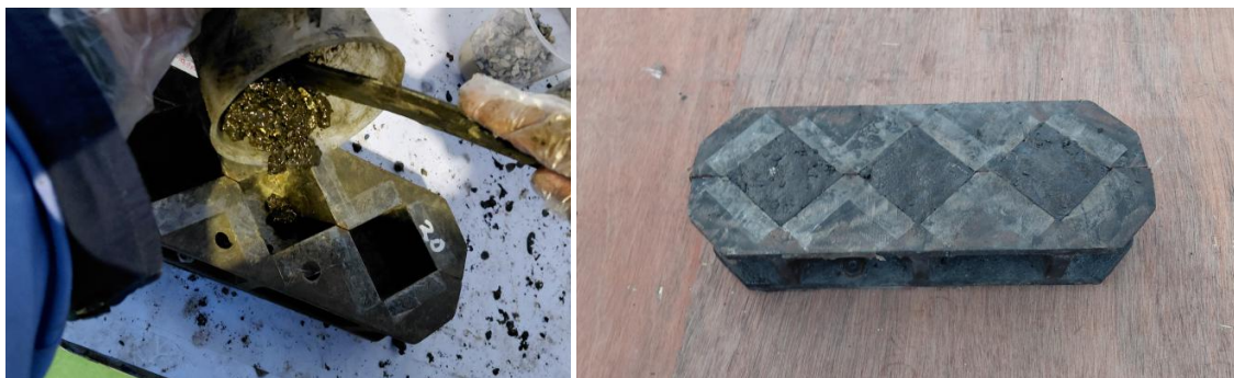
Figure 2. Mixing of Polymer Concrete (Left) and Condition of Concrete After Curing (Right)
