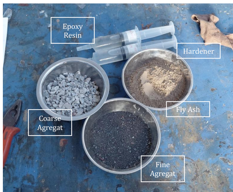
Figure 1. Constituent Materials of Polymer Concrete
