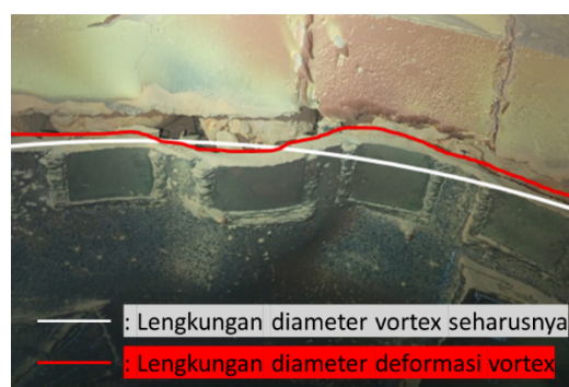
Figure 3. Deformation on the Vortex Finder Surface
