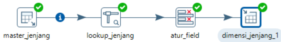
Figure 3. ETL Design for the Level Dimension
