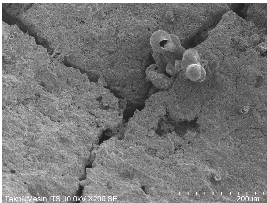
Figure 12. Appearance of Chromium Carbide Precipitate in Material A
